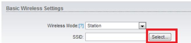
7.) A new screen will pop up and a Site Survey will be carried out. This means that the antenna is scanning for wireless networks and will report back as to what it has been able to detect in the direction the antenna is facing. The screen (*pictured below*) reports the name of the network (SSID), the type of encryption used (if the network does not require a password, this will be listed as 'None') and the strength of the signal.
