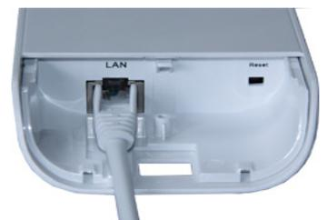
Ensure all of the components are connected together before connecting the power cable to your 12v supply.
