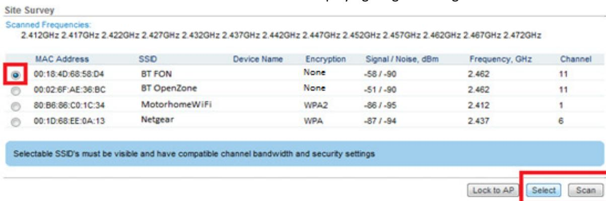
8.) You may find it helpful at this point to hand hold the antenna either up through a rooflight, out through a window or windscreen or temporarily mount it if you wish. You may adjust the antenna in any direction and press **SCAN** (bottom right) at any time which will re-scan the available networks. As you adjust the antenna you will notice that some networks appear and disappear and the signal strength will alter.
