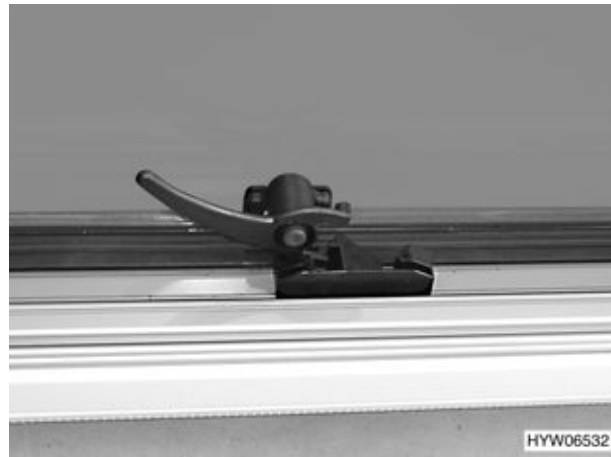
Fig. 42 Hinged window, window handle in the "continuous ventilation" position (variant 2)
