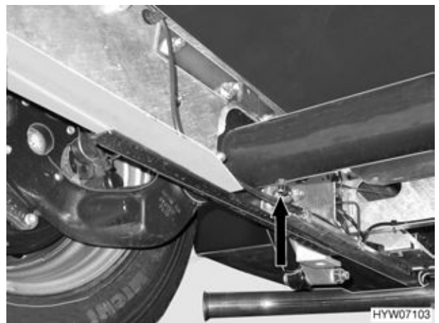
Fig. 191 AL-KO rear axle
