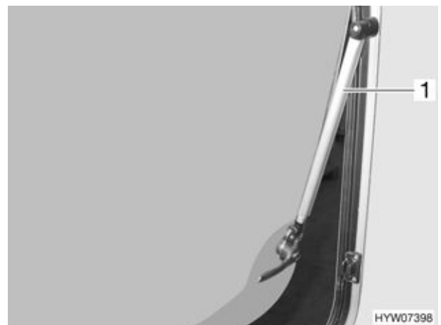
Fig. 44 Hinged window, telescopic rod (variant 3)
