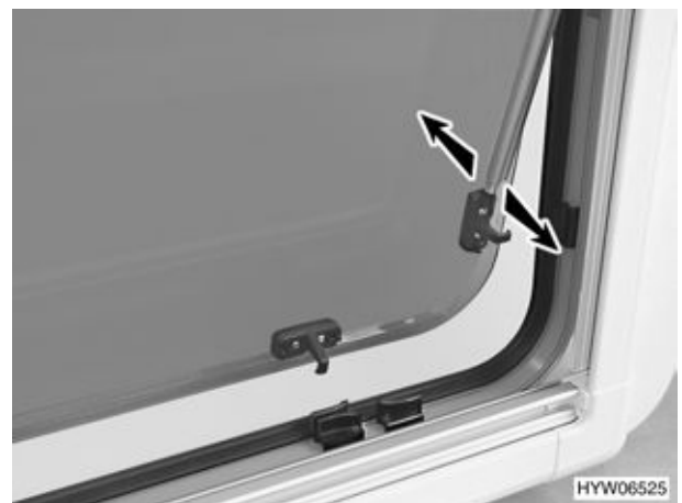
Fig. 40 Hinged window, telescopic rod (variant 2)
