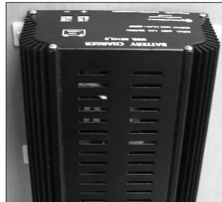
(c) Charger/ Transformer Unit
