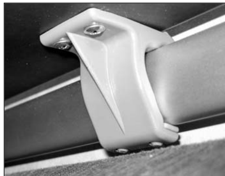
To lock the table, raise the table 45°, push clip to rail and lower table.
