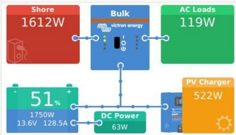
**ESS Mode is *Keep batteries charged*. Shore power is being tapped to recharge batteries as quickly as possible.**
