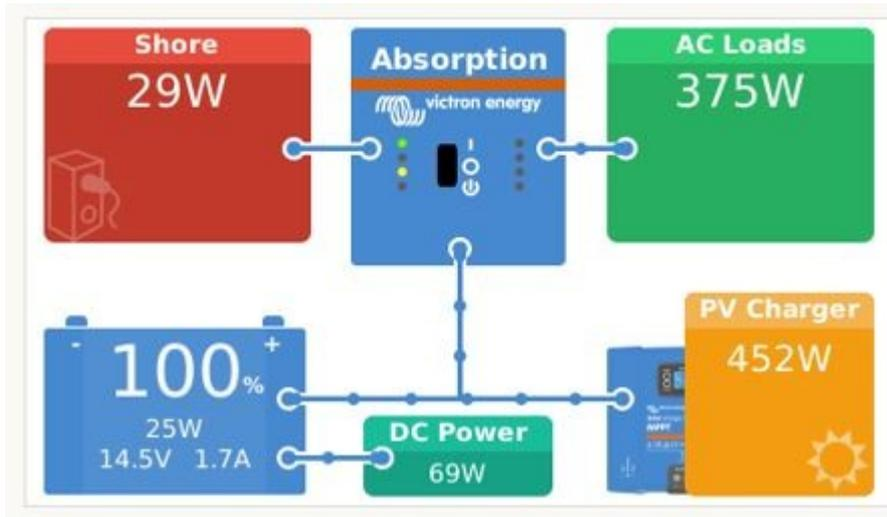
ESS Assistant loaded and mode is **Optimized (without Battery Life)**. **Grid setpoint = 30W**. The **PV Charger** is supplying all required power to trailer as available  $PV \geq AC\ Loads + DC\ Power$
