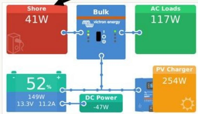
**Grid setpoint 40W.** This keeps the shore power connection “alive” even when there is sufficient PV power. I chose 40W...could be more, could be a bit less.
