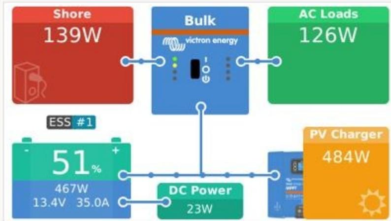
Battery SOC (51%) is near **Minimum SOC (unless grid fails)** setting (50%), so state is **ESS #1**. **AC Loads** supported by **Shore** power. **PV Charger** power going to batteries.
