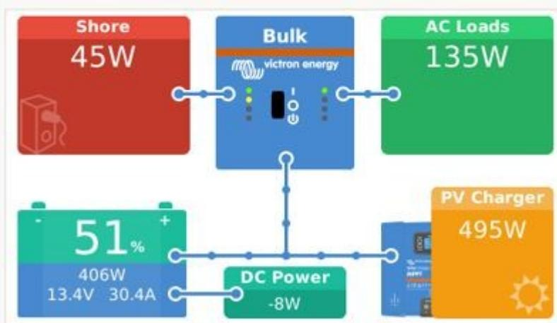
**Minimum SOC** setting is 25%. **AC Loads** and **DC Power** supported by **PV Charger**.
