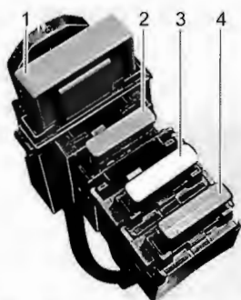
Fig. 68 Fuses (living area battery)
